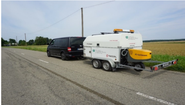
2.6 pav. ViaTech AS kelio analizatorius ir rašytuvas (CEN/TS 15901-14:2016) Fig. 2.6. Road Analyser and Recorder of ViaTech AS (CEN/TS 15901-14:2016)
