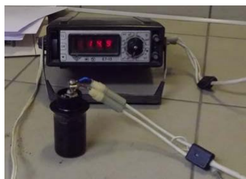
Fig. 4. Equipment used for measuring electrical capacitance
