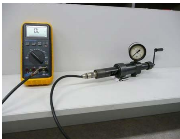
Fig. 2. Equipment for measuring electrical resistance of char
