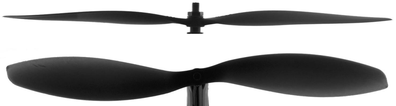
1.8 pav. Propeleris APC Slow Flyer 11x4,7 (UIUC, 2015)
