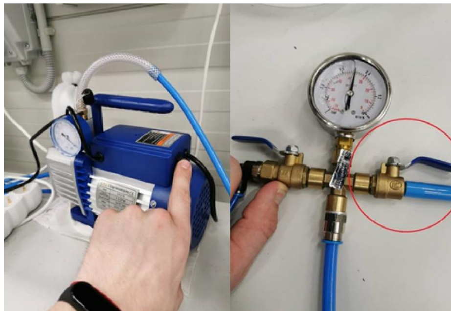
Fig. 23. Air pump and valve with pressure indicator
