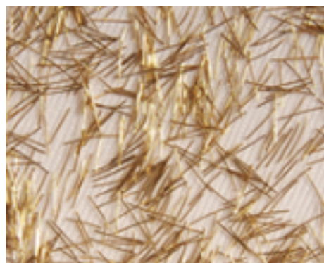
2 pav. Plieninis mikroplaušas (Fibrezone, Micro Steel Fibre Brass Coated, 2019)
