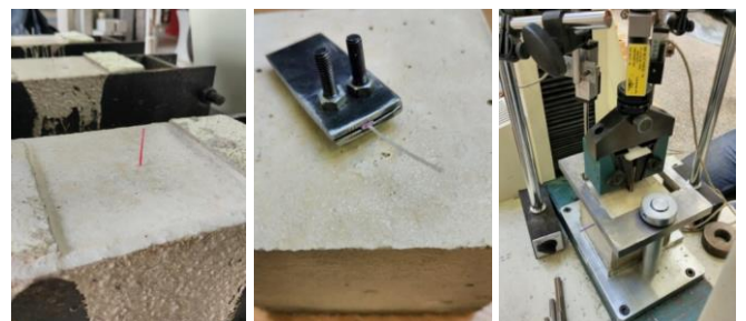
Figure 3. Test preparation: fiber protected with a plastic sleeve (left), steel clamps (middle), testing machine (right)
