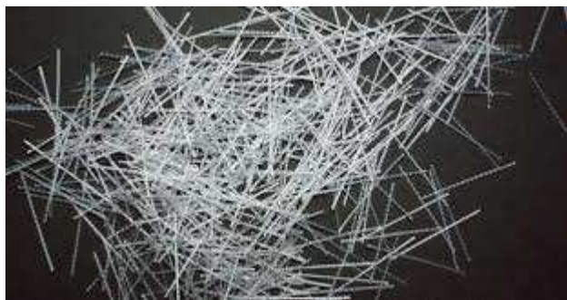
1 pav. Sintetinis makroplaušas ( GCP Applied Technologies Inc., 2017)
