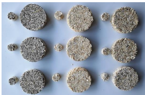
Fig. 1. Sound absorption samples (from left: HW; W; H)
