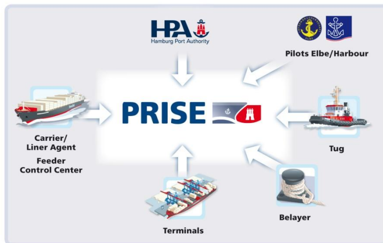
Figure 7-3: Port River Information System Elbe – PRISE
