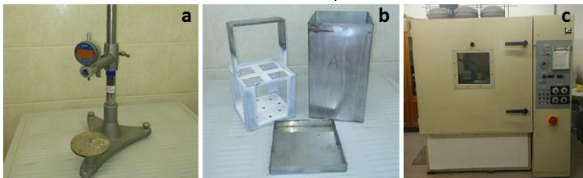
Figure 1. Used equipment: a- Digital dial indicator and frame; b- Stainless steel container; c- Climatic chamber
