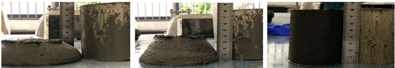
Figure 13. Buildability assessment of 3D printed concrete with sand of different fineness [56].
