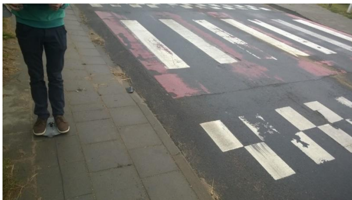
Fig. 2.6 Steel plate and accelerometer use in field measurements
