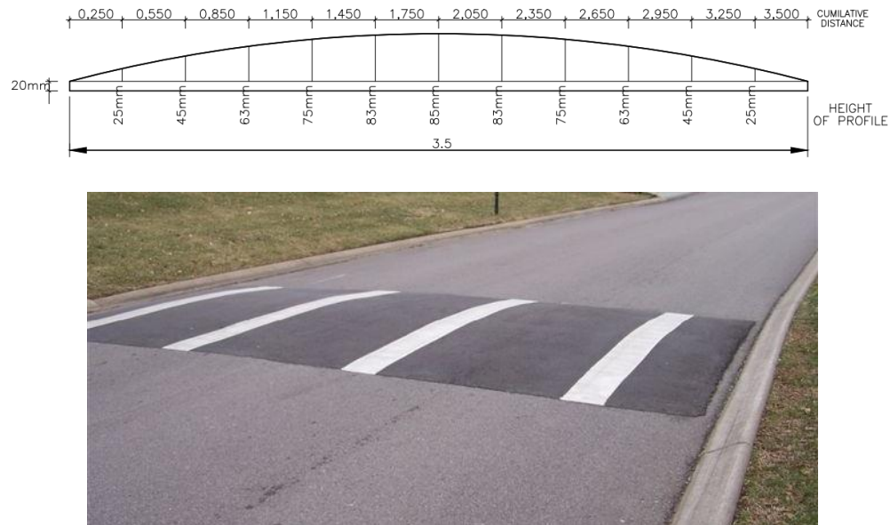
Fig. 1.11 Typical speed hump (City of Tshwane, https://brentwood-tn.org )
