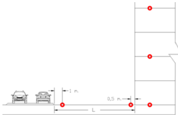
Fig. 2.7 Principal scheme of vibration measurement points (method A)
