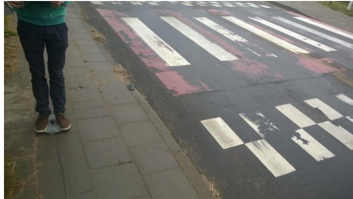
Fig. 3. Steel plate and accelerometer use in field measurement (author's picture)
