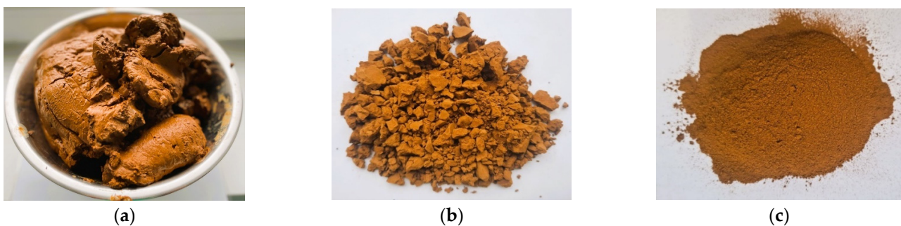
Figure 3. Drinking water treatment sludge (DWTS): (a) raw; (b) dried; (c) dried/milled.
