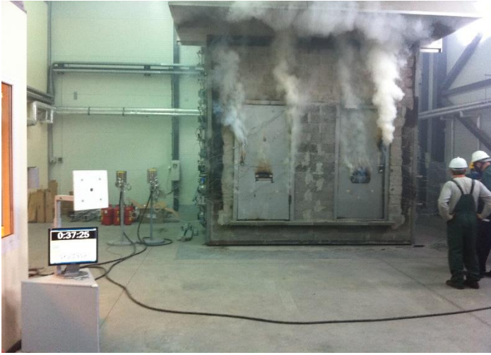
Fig. 5. Scheme of investigated multilayer structure (a) and photography of the wall with specimens fastened to the furnace (b) and fire tests (c): 1–26 – temperature measuring points; D1–D11–thermal displacement measuring points
