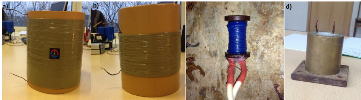
Fig. 25. Designed inductors that will be used for magnetic flux density analyses in the center of them. a) Inductor X, b) Inductor Y, c) Inductor Z, d) Inductor W
