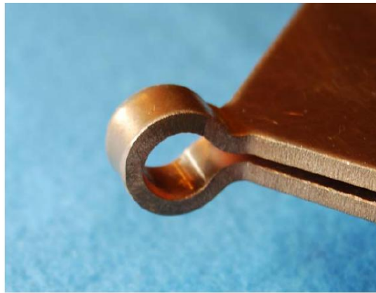
Fig. 5. Two-megagauss single-turn inductor design, courtesy C. Mielke, LANL. [13], [8]
