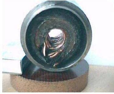
Fig.10. Destructed pulsed solenoid [5]
