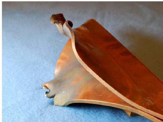
Fig. 6. Same inductor assembly after a shot, courtesy C. Mielke. [13], [8]
