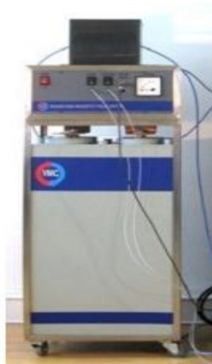
Fig. 34. Capacitor bank used in experiments with 5.4 mF
