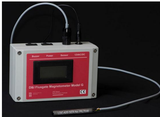
1.12 pav. Fluxgate daviklio imtuvas ( http://www.mingeo.com/ 2014)
