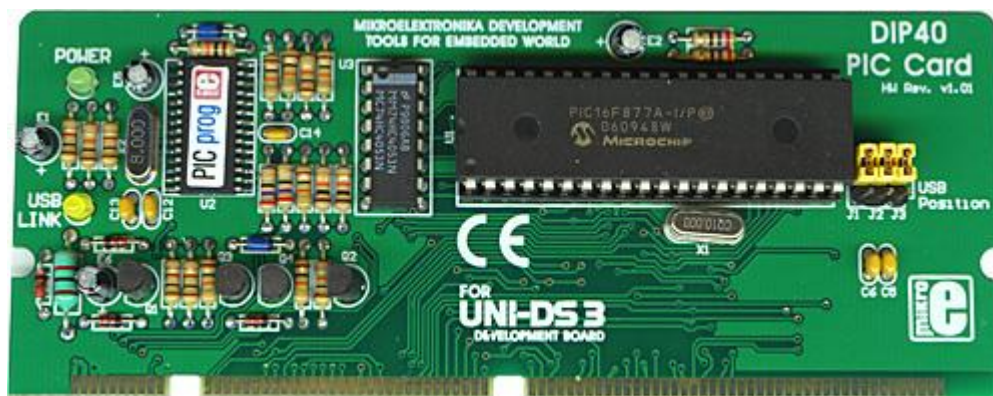
4.14 pav. PIC16F877A mikrovaldiklis
