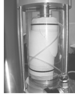
Fig 3. Triaxial test sample with free horizontal movement of sample base
