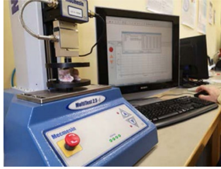
Fig. S2.2. Compression of the dog's lumbar vertebra
