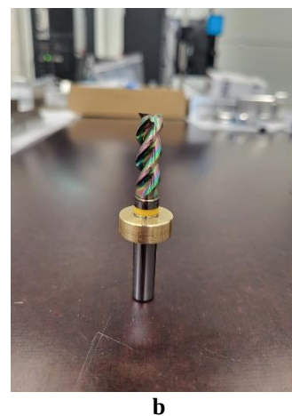
Fig. 3 Sketch (a) and image (b) of the end mill used to machine a vertical wall
