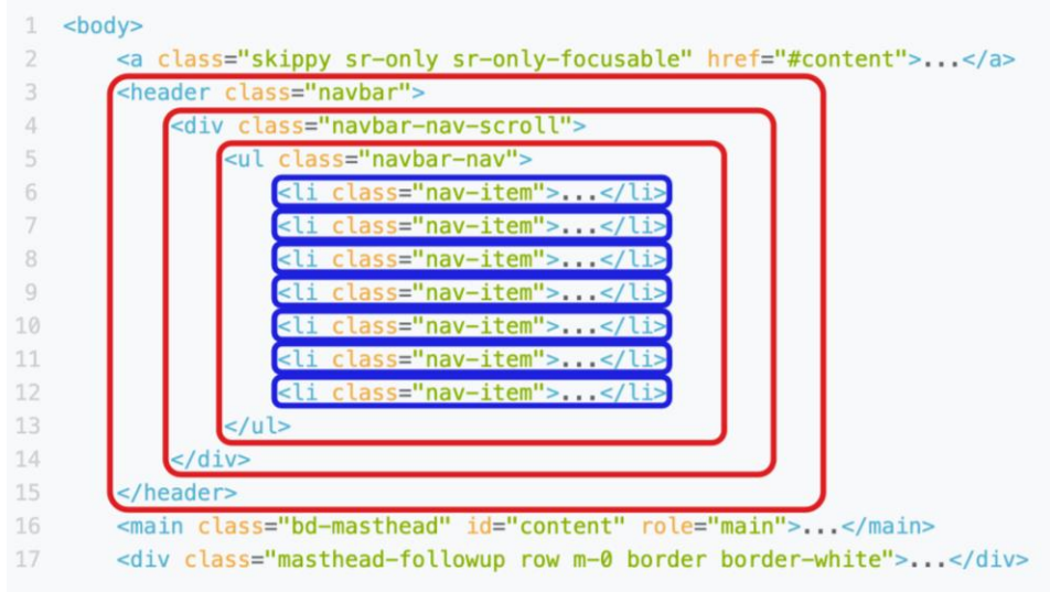
Fig. 3.2. Example of HTML block variations where red blocks can be considered containers and all three cases can be assumed as correct bounds of the block
