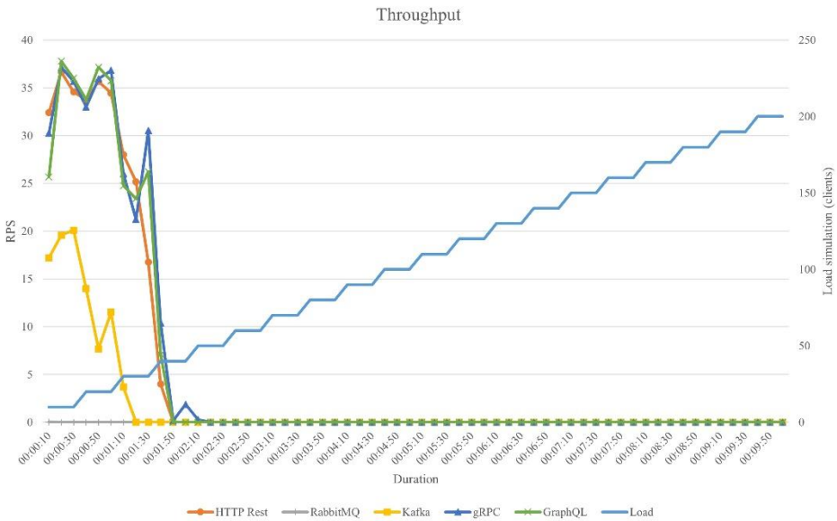
Fig. 3.19. Throughput test results for 10,000,000-character-size messages
