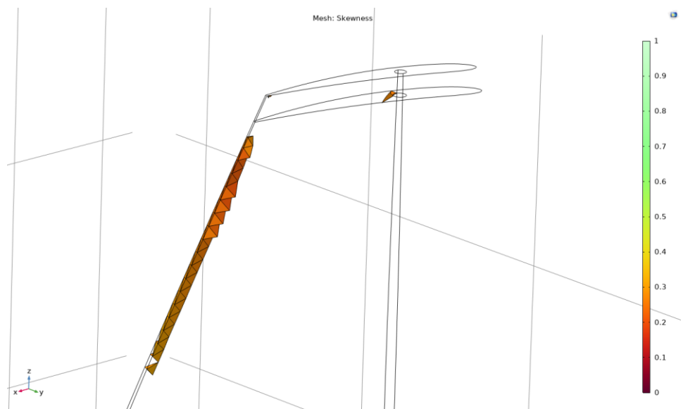
Fig. 2.10. Elements quality < 0.3 at the tip of the blade (prepared by author)
