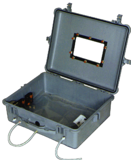
Fig. 2.3. Vacuum chamber with integral pump
