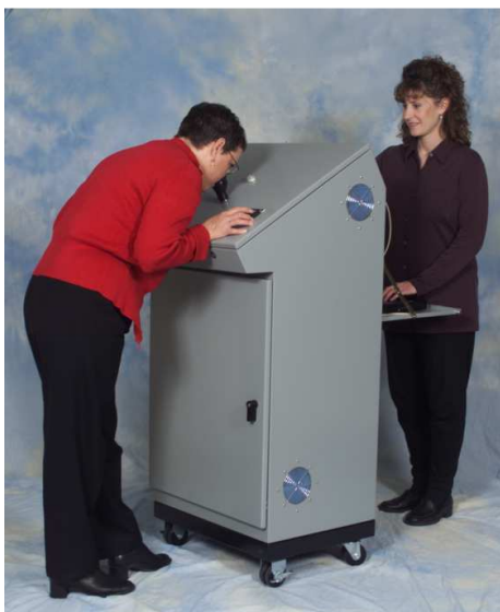
Fig. 2.4. AC'SCENT International Olfactometer with the test administrator and the assessor (St. Croix Sensory 2005)
