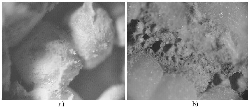
Fig. 5. Macrostructure of composite material (enlarged by 25 times): a) sample with density of 150 kg/m 3 ; b) sample with density of 350 kg/m 3
