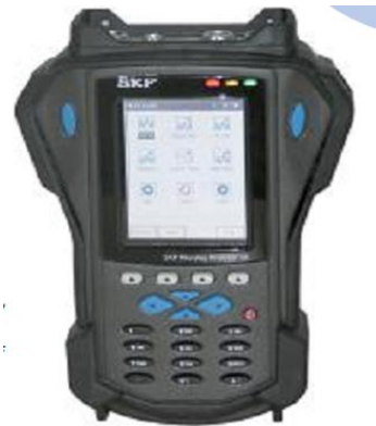
38 pav. SKF Microlog Analyzer GX series CMXA 75
