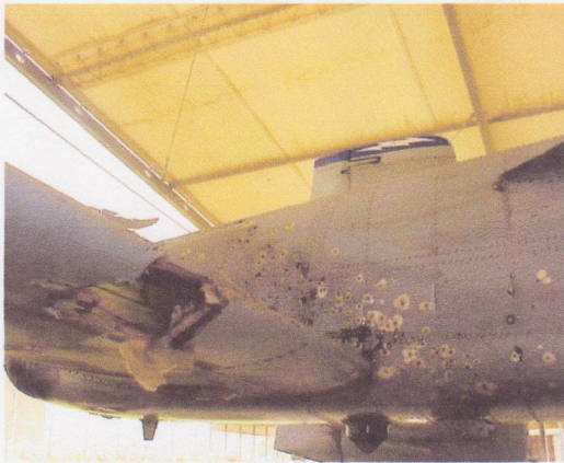
Fig. 4. An A-10 military aircraft hit by numerous number of small-arms fire.
