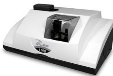
2.2 pav. „Cilas Particle Size Analyzer 1090“ lazerinis granuliometras (Directindustry, 2023)
