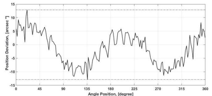
Fig. 5. Averaged position deviation plot of both optical sensors.
