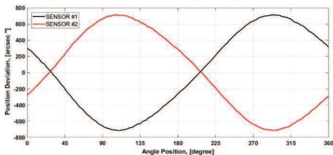
Fig. 4. Calibration chart of the developed encoder prototype: position deviation of sensor #1 (black line); position deviation of sensor #2 (red line).
