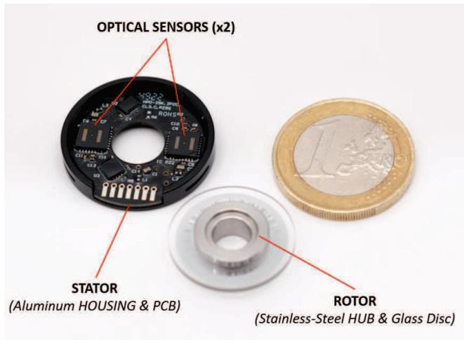
Fig. 1. View of developed modular optical encoder kit.
