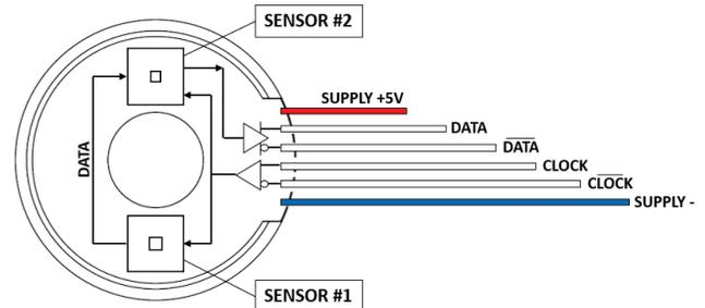
Fig. 3. The principle electrical scheme of the encoder.
