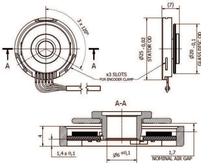
Fig. 2. Mechanical drawing with main dimensions of the encoder.
