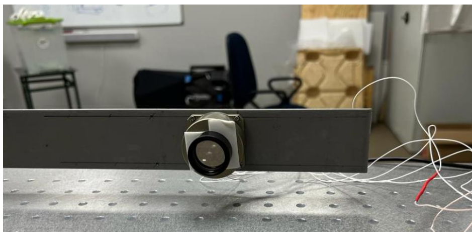
Figure 35. Mirror attached to the reaction wheel.
