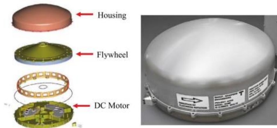
Figure 3. Reaction wheel structure (Sensel....2012)
