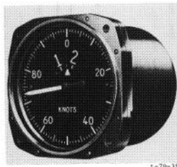
Figure 12. Airspeed indicator (Technical Order Overhaul Instructions - Sensitive Airspeed Indicator, 1967)
