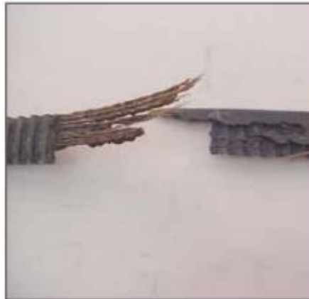
Figure 1.3.4 Normal belt failure example
