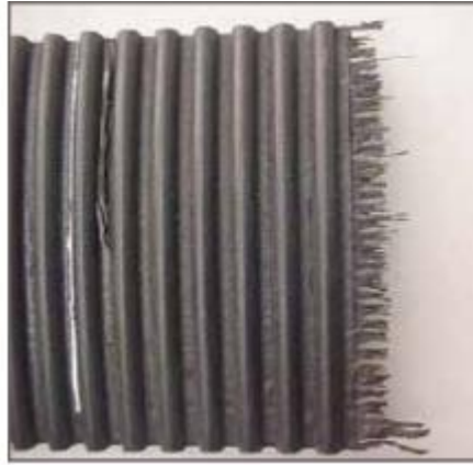
Figure 1.3.5 Crimp failure example
