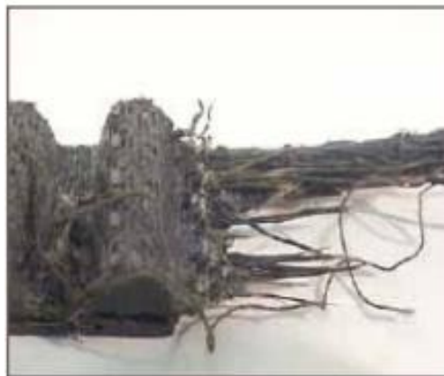
Figure 1.3.6 Shock load failure example
