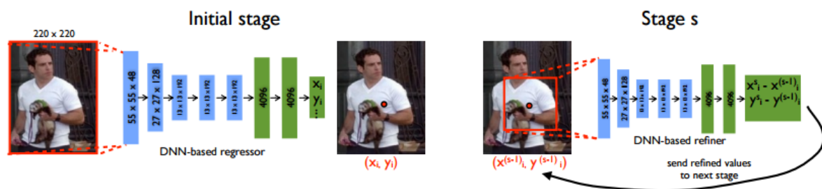
Figure 3-3: CNN-based regressor and refiner architectures [16]
