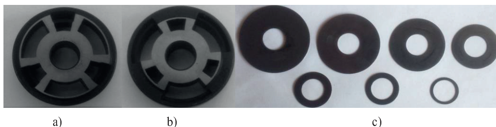
Fig. 2 Parts of the researched shock absorber: a - piston compression side; b - piston rebound side; c - samples of the valve shims used for tests
