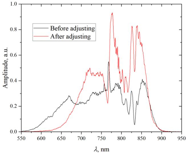
**Fig. 7:** Difference in spectrum shape before and after adjusting the fiber. The spectra are related to transverse modes shown in Figure 6.
