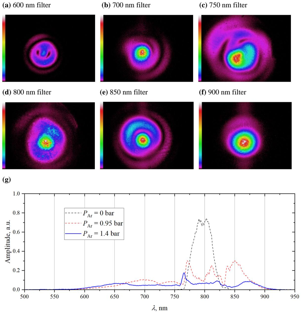
**Fig. 12:** Images (a) – (f) depict transverse modes with all the light filtered except for a denoted wavelength. The graph (g) visualizes spectra at vacuum and two different pressures. The images of the modes are related to spectrum which is visualized as a solid curve ( $P_{\text{Ar}} = 1.4 \text{ bar}$ ). The focal distance of the lens is 2.5 m.
