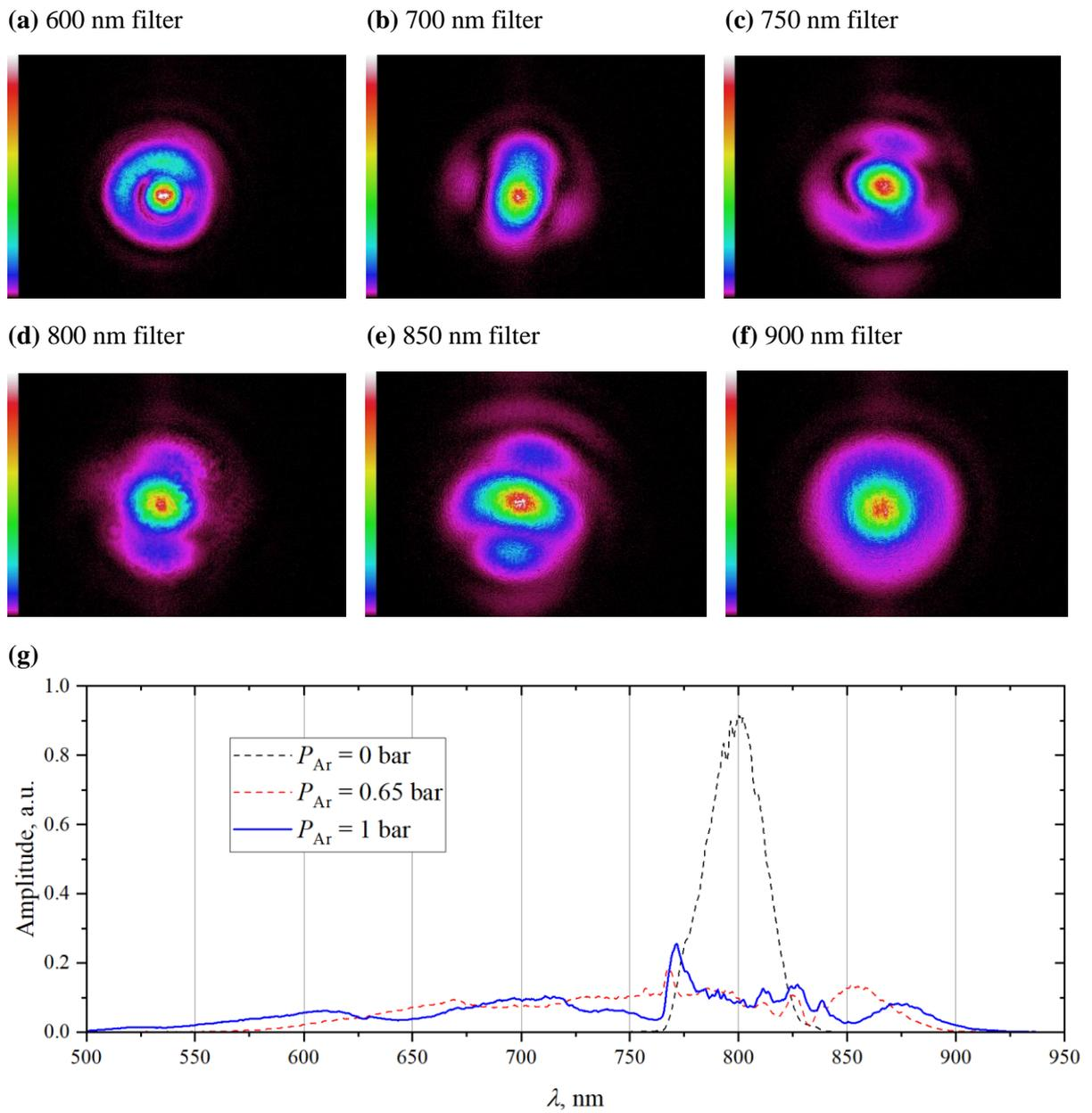
**Fig. 10:** Images (a) – (f) depict transverse modes with all the light filtered except for a denoted wavelength. The graph (g) visualizes spectra at vacuum and two different pressures. The images of the modes are related to spectrum which is visualized as a solid curve ( $P_{\text{Ar}} = 1 \text{ bar}$ ). The focal distance of the lens is 2 m.
