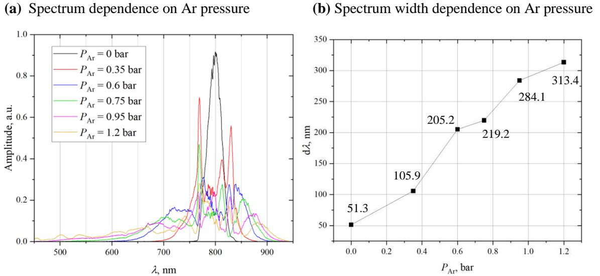
**Fig. 5:** Spectrum dependence on the Ar pressure inside the hollow-core fiber. Graph (a) depicts the spectra at each pressure value, showing the change in width and different peak values. (b) demonstrates the linear dependence of spectrum width on the pressure, the width is measured at the peak/ $e^2$ , since there is no central wavelength at higher pressures, instead, different peaks separated by 50 nm and more, so the FWHM would not determine the full width of the spectrum.
