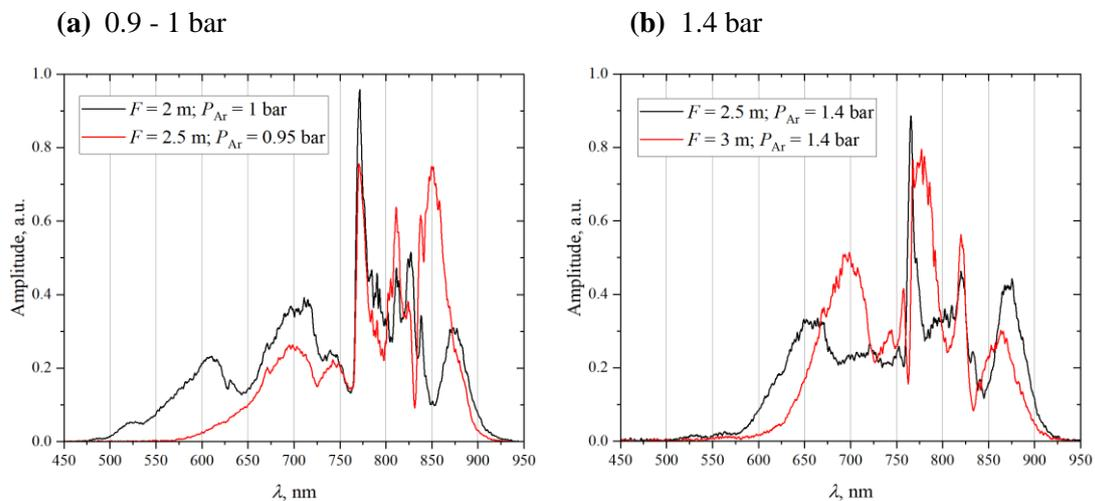
**Fig. 16:** Spectra measured at similar pressures, having different lenses installed.
