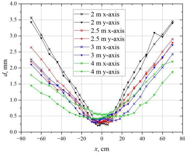
(b) Transverse mode size dependence on the distance from a focal point (scaled)
