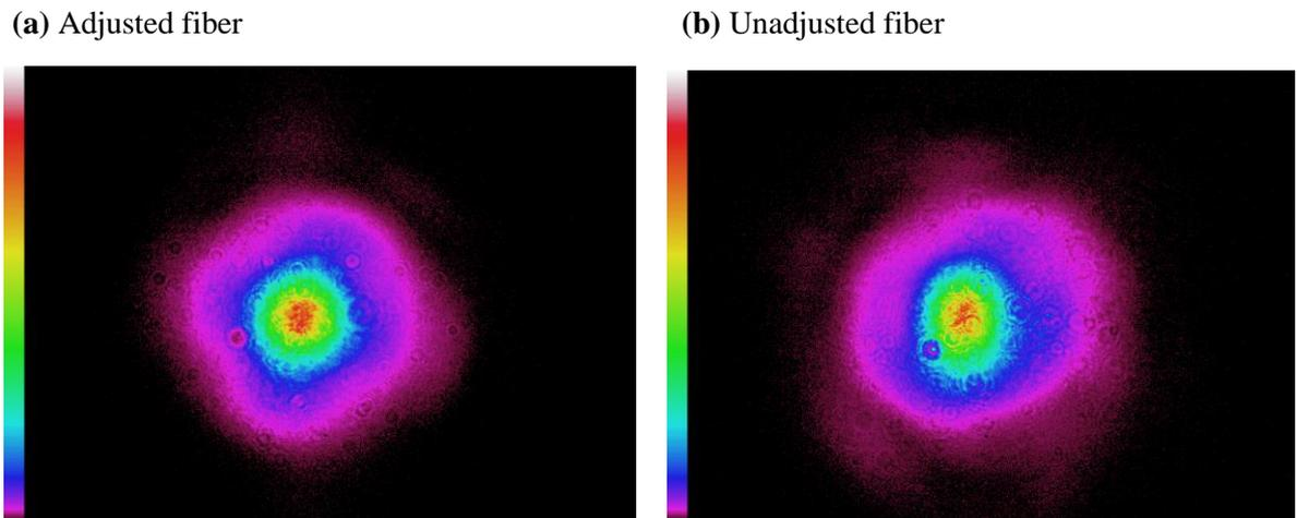
**Fig. 6:** (a) Transverse mode after adjusting the fiber ends at  $P_{Ar} = 0.65$  bar;  $x = 1.311$  mm,  $y = 1.316$  mm; 2-meter focal distance lens equipped. (b) Image taken from Figure 4;  $x = 1.223$  mm,  $y = 1.496$  mm. (c). The pressure difference of 0.05 bar is too negligible to deform the mode, so (a) and (b) are comparable.
