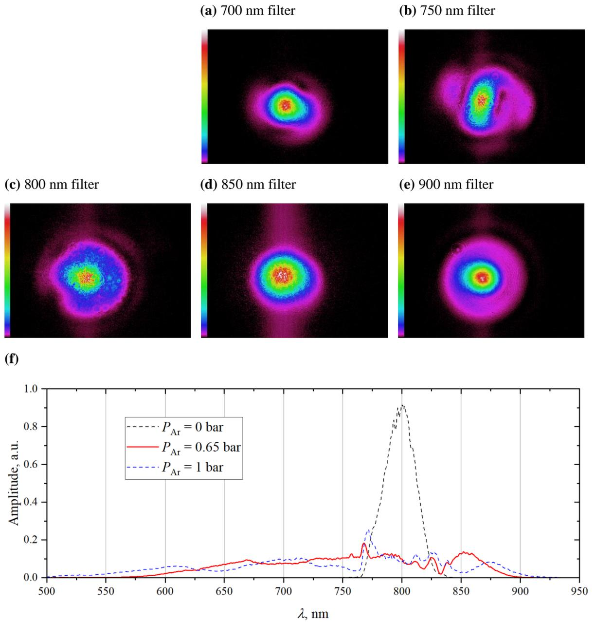
**Fig. 9:** Images (a) – (e) depict transverse modes with all the light filtered except for a denoted wavelength. The graph (f) visualizes spectra at vacuum and two different pressures. The images of the modes are related to spectrum which is visualized as a solid curve ( $P_{Ar} = 0.65$  bar). The focal distance of the lens is 2 m.
