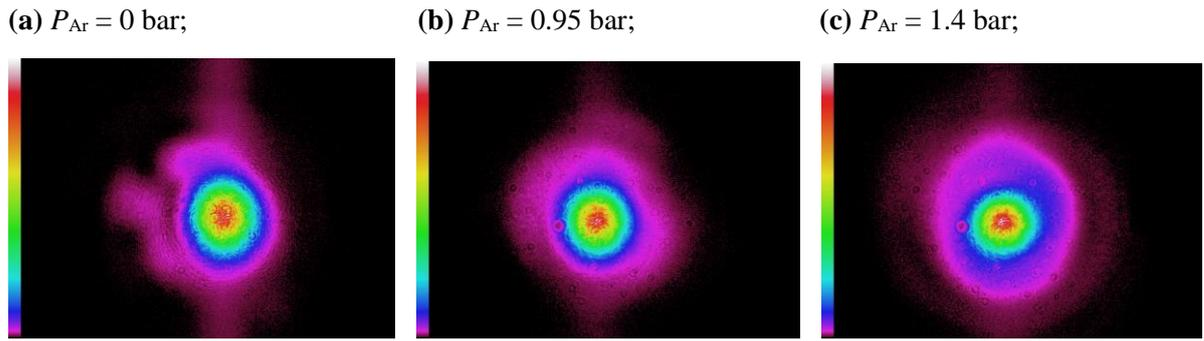
**Fig. 14:** Transverse mode images,  $F = 2.5$  m lens. (a)  $x = 1.342$  mm,  $y = 1.540$  mm;
