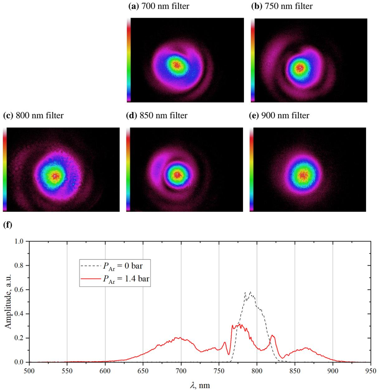
**Fig. 13:** Images (a) – (f) depict transverse modes with all the light filtered except for a denoted wavelength. The graph (g) visualizes spectra at vacuum and pressures of 1.4 bar (The pressure inside the hollow-core fiber should not exceed 1.5 bar to prevent its damage). The images of the modes are related to spectrum which is visualized as a solid curve ( $P_{Ar} = 1.4$  bar). The focal distance of the lens is 3 m.
