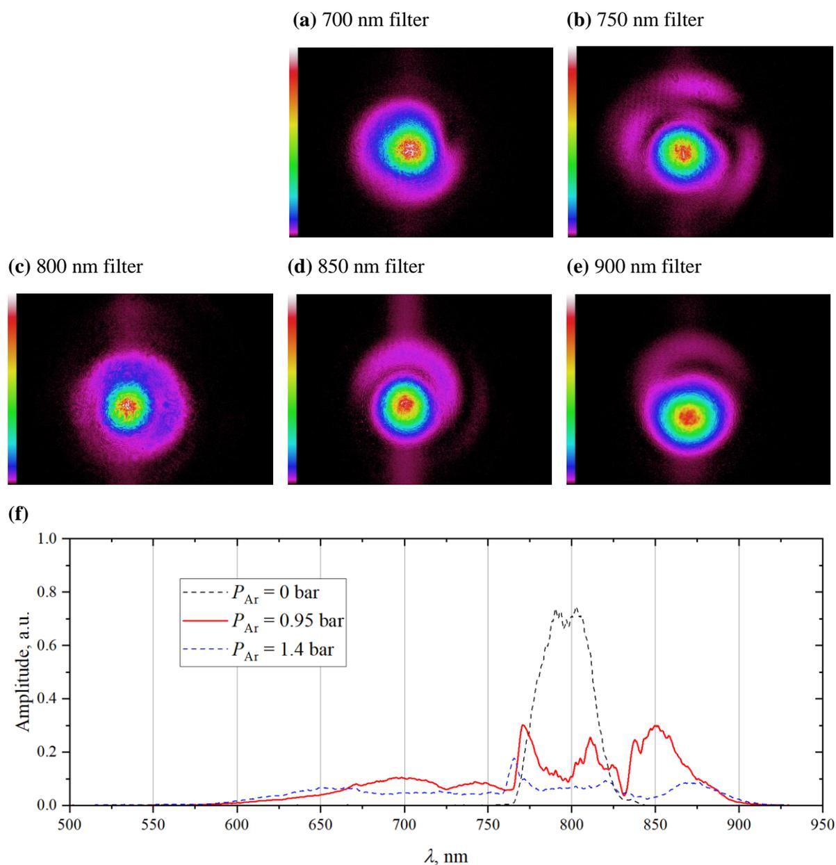
**Fig. 11:** Images (a) – (f) depict transverse modes with all the light filtered except for a denoted wavelength. The graph (g) visualizes spectra at vacuum and two different pressures. The images of the modes are related to spectrum which is visualized as a solid curve ( $P_{Ar} = 0.95 \text{ bar}$ ). The focal distance of the lens is 2.5 m.
