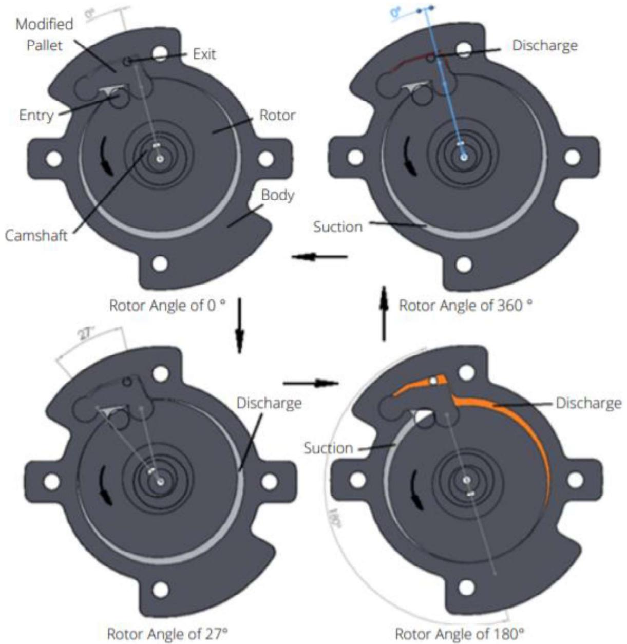
*Fig. 4. Suction- Discharge phase concerning the rotor angles
