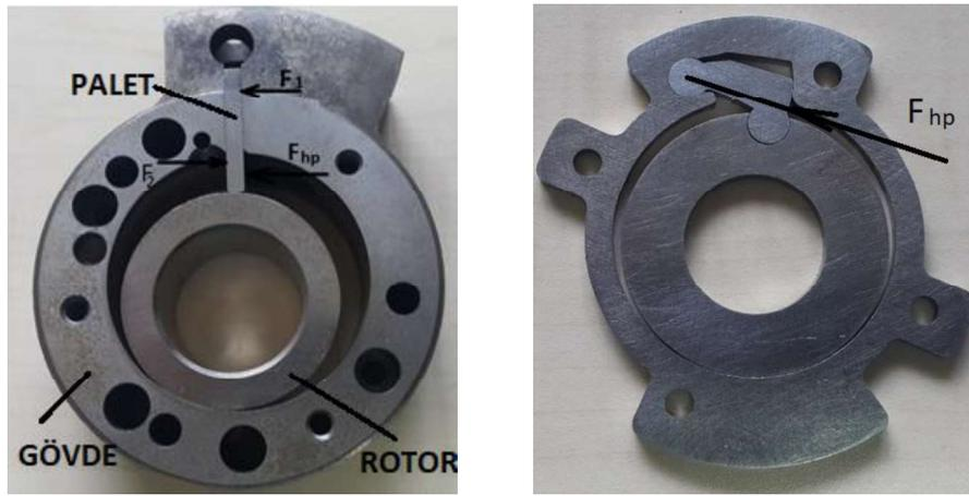
**Fig. 2.** Classical and Novel vane Designed Compressor Body, Rotor, and Palet
