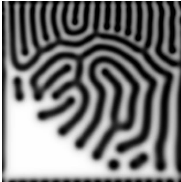
Figure 10. Reaction-diffusion model parameter scan: Diffusion A=scan on X-axis 0.6 to 1.1; Diffusion B=scan on Y-axis 0.25 to 0.75; feed of A=0.029; kill of B=0.057
