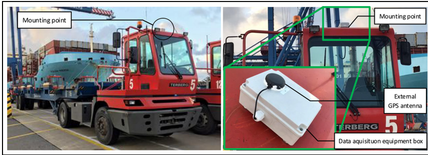
Figure 5. Example of the trucks used in the experiment and the selected mounting point on the vehicle.
