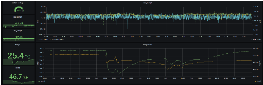
Figure 54. Sensor data transfer experimental study using LoRaWAN (temperature and humidity).
