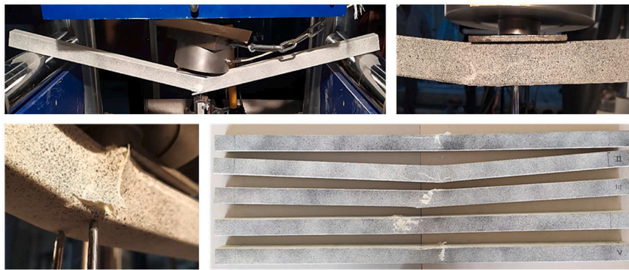
Fig. 4. The bending specimens' failure.
