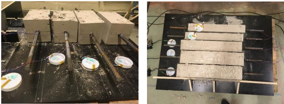
Fig. 2.10. Pictures of the DOFS-instrumented RC ties
