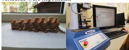
a) b) Figure 1: a) Spayed dog vertebrae (Th11-L5) b) Mecmesin MultiTest 2,5-i microcompression machine.
