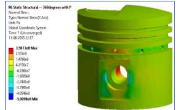
Fig 5.58 Si 3 N 4 Normal stress with combustion pressure @ 360°C
