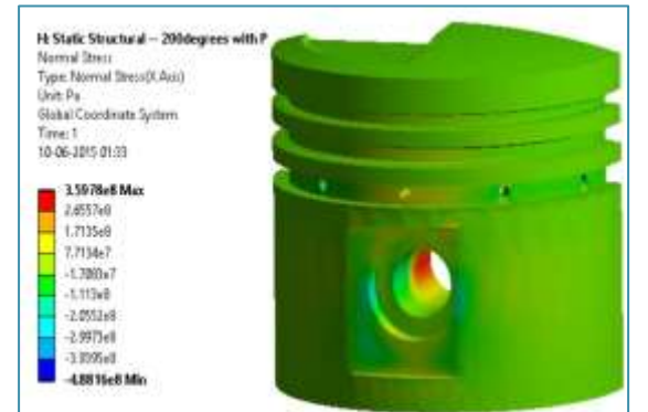
Fig 5.56 Si 3 N 4 Normal stress with combustion pressure @ 200°C
