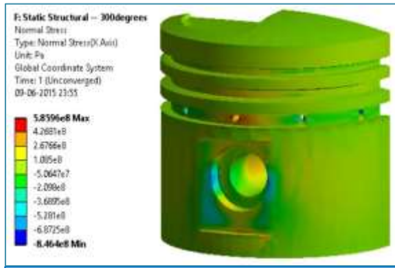
Fig 5.51 ZrO 2 Normal stress without combustion pressure @ 300°C
