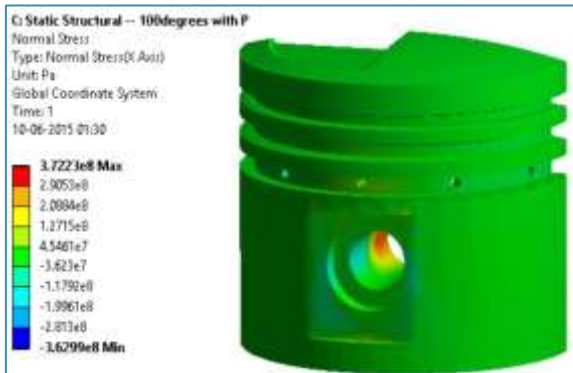
Fig 5.55 Si 3 N 4 Normal stress with combustion pressure @ 100°C
