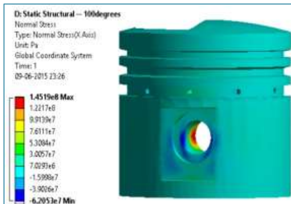
Fig 5.38 Al 413.0 Normal stress without combustion pressure @ 100°C
