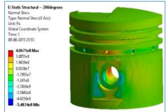
Fig 5.50 ZrO 2 Normal stress without combustion pressure @ 200°C
