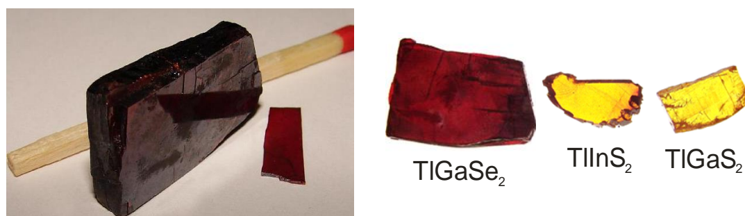
Fig. 1.1 (left) TI GaSe 2 slab and a sliced thinner sheet of d = 200 \mu\text{m} in comparison to 5 cm long match; (right) three layered semiconductors TI GaSe 2 (same as in the left), TI InS 2 , and TI GaS 2 with a characteristic absorption band of 2.14 eV, 2.34 eV and 2.64 eV, respectively. The band edge energy determines the color of the subband transmitted light.
