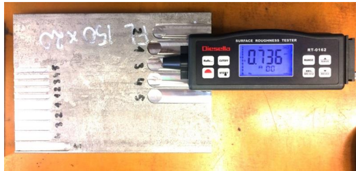
Fig. 2.10. Milled surface roughness measurements procedure
