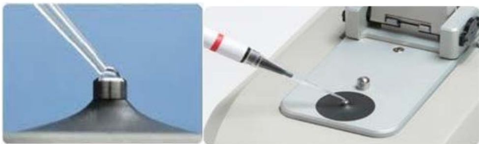
Fig. 2.2.3.1. Evaluation of DNA concentration and purity by spectrophotometer „Nanodrop 2000“ (Isogen Life Science, 2012)
